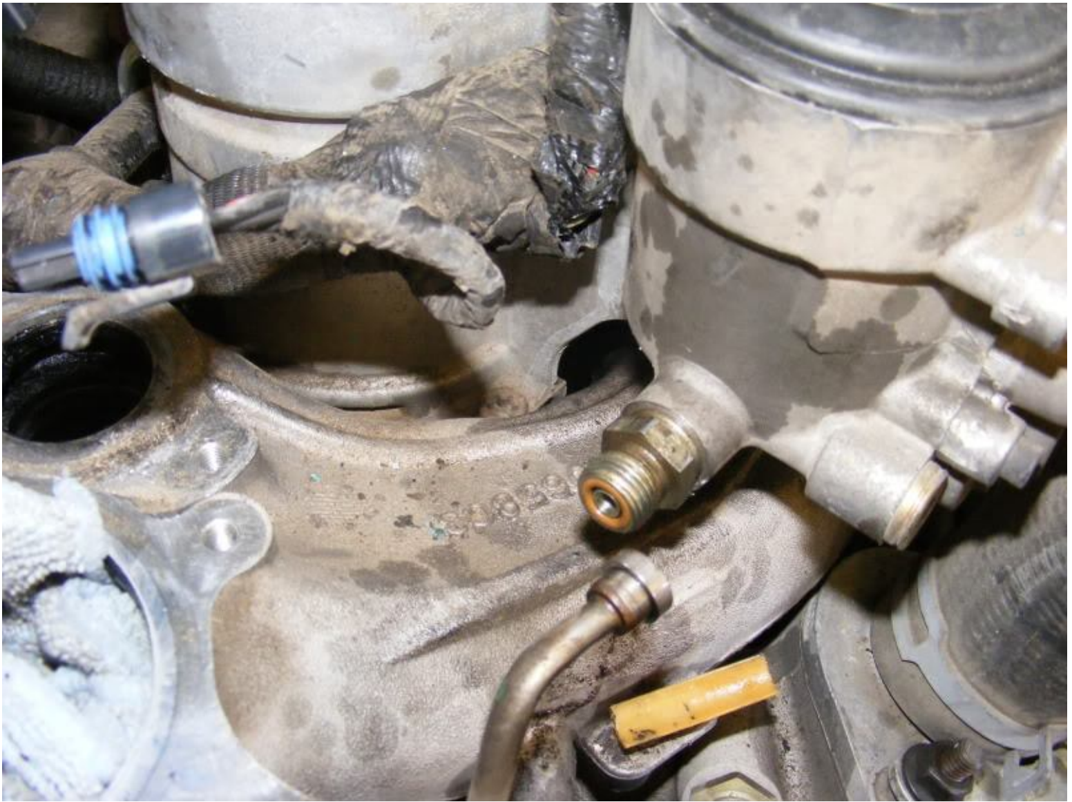
Fuel lines: Notice the line in the front (this is the one that required 2 wrenches)
