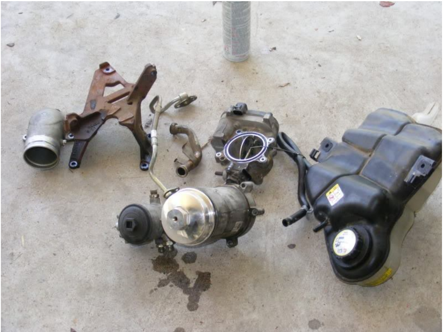
Here is a few of the parts that was removed before the cooler could come off: Left to right (Intake Elbow, Turbo Bracket, Turbo Oil Line, Throttle Plate, Coolant over fill, Oil and fuel filter housings)
