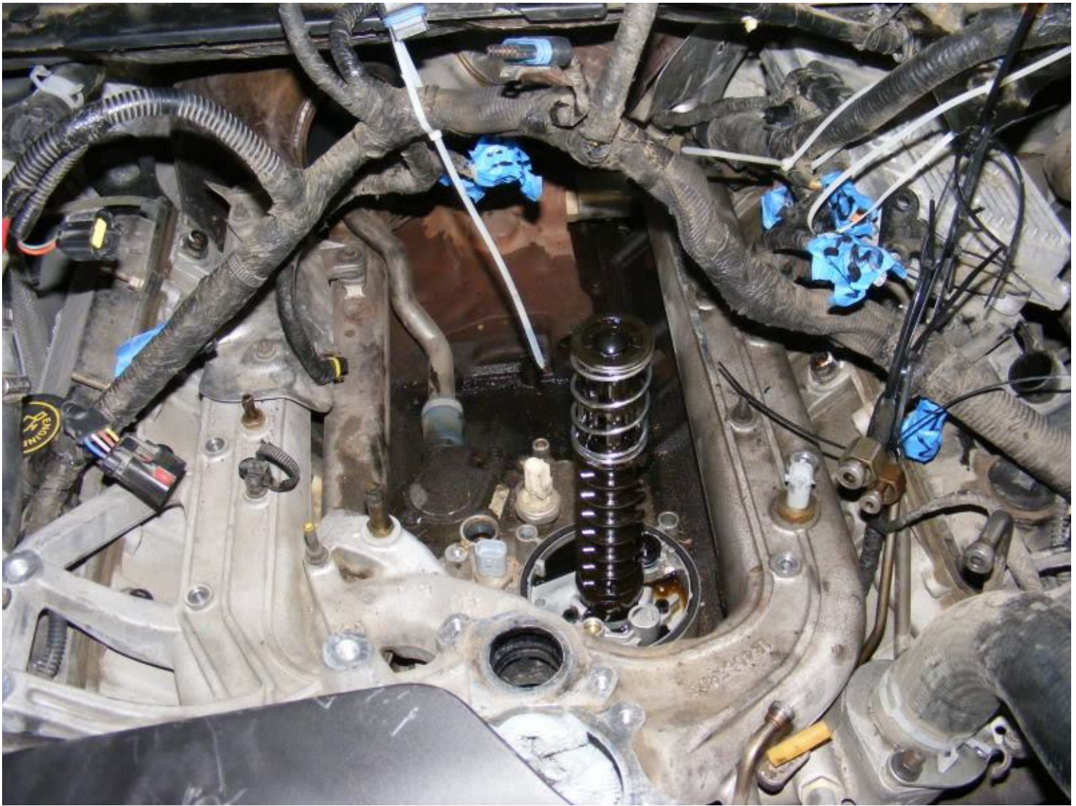
Here you can see the engine harness zip tied out of the way for easy access to the intake plenum.
